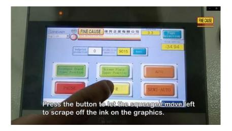
Press the button on the <u>screen printer</u> to let the squeegee move left to scrape off the ink on the graphics.
